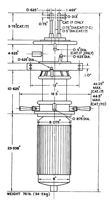
Filament Starting. The cold resistance of the filament is of the order of  $0.0057~\Omega$ . The filament current must never exceed 500 A at any time during the switching-on period. If the valve is operated for periods greater than 15 minutes without anode voltage being applied, the filament voltage must be reduced to one-half its normal value during the standby period.
