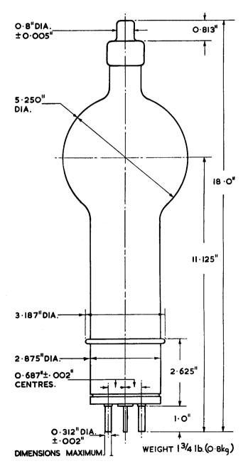
the rectifier must not be fitted into a tube nor must any obstruction be allowed to impede the free air circulation around the valve.
