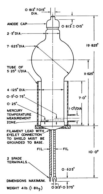
The blower must be switched off for ambient temperatures between 10°C and 25°C, and on for temperatures between 25°C and 45°C. The valve must never be operated when the ambient temperature is below 10°C. For condensed mercury temperatures below 30°C and above 40°C the peak inverse voltage must not exceed 10,000 volts. The equilibrium condensed mercury temperature rise above ambient temperature at full load is approximately 15°C.
