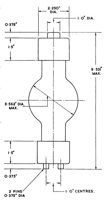
Filament Adjustments. The life of the rectifier is governed to a great extent by the operating temperature of the filament. In order to obtain long life, the practice of energizing the filaments just before the radiographic exposure, and turning them off immediately thereafter, should be followed.
