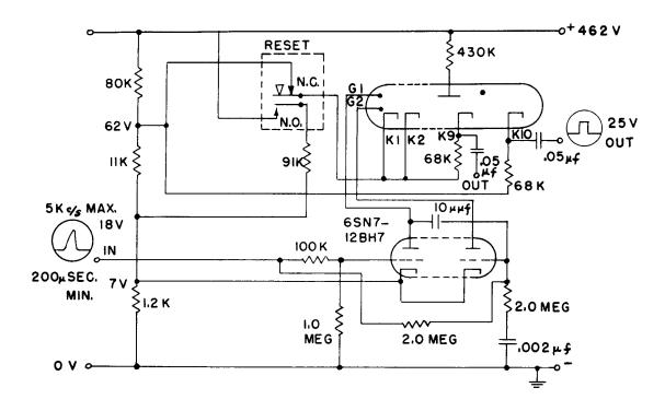
6476 GLOW TRANSFER COUNTER TUBE DRIVER CIRCUIT
