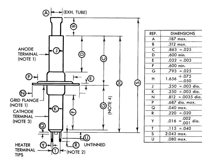
Note 1: Maximum allowable eccentricity of anode terminal or grid flange with respect to cathode terminal is .008 in. measured .080 in. from end of anode and cathode. Tube to be chucked .050 in. to .100 in. from the cathode flange.
