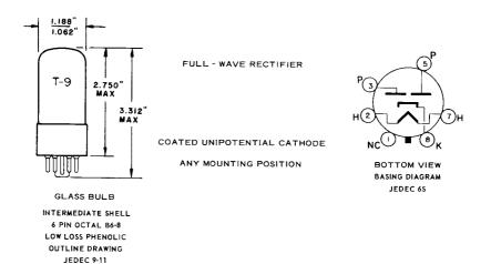
THE 6X5WGT IS A CATHODE TYPE FULL-WAVE RECTIFIER EMPLOYING A T-9 ENVELOPE WITH A LOW LOSS OCTAL BASE. IT IS DESIGNED FOR USE IN APPLICATIONS WHERE SEVERE CONDITIONS OF VIBRATION AND SHOCK ARE ENCOUNTERED.
