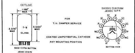
THE TUNGSOL 34CD3 IS AN INDIRECTLY-HEATED DIDDE IN COMPACTRON CONSTRUCTION. IT IS INTENDED FOR USE IN DAMPER SERVICE OF TELEVISION HORIZONTAL DEFLECTION CIRCUITS. IT IS DESIGNED TO WITHSTAND HIGH VOLTAGE PULSES BETWEEN CATHODE AND BOTH HEATER AND PLATE ELEMENTS SUCH AS NORMALLY ENCOUNTERED IN "DIRECT DRIVE" CIRCUITS. ITS HIGH CURRENT CAPABILITY MAKES IT PARTICULARLY SUITABLE FOR COLOR TELEVISION APPLICATIONS.
