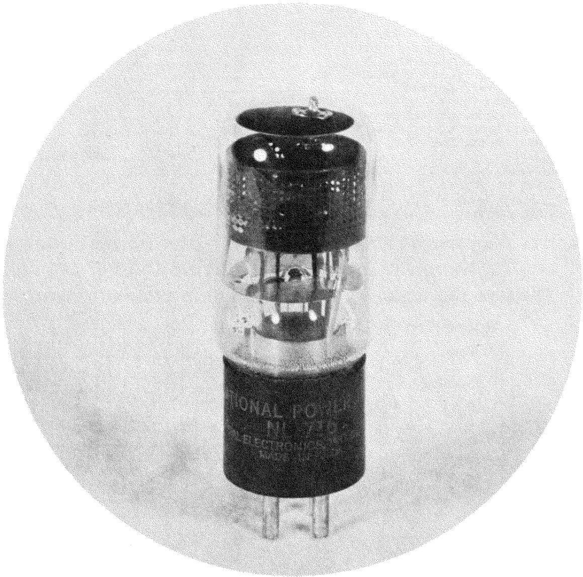
NATIONAL POWER TUBE NL-716 is a compact, quick heating thyratron designed for timing and control applications. It is gas and mercury filled for quick starting and wide temperature limits. NL-716 gives long life without circuit cushioning.
