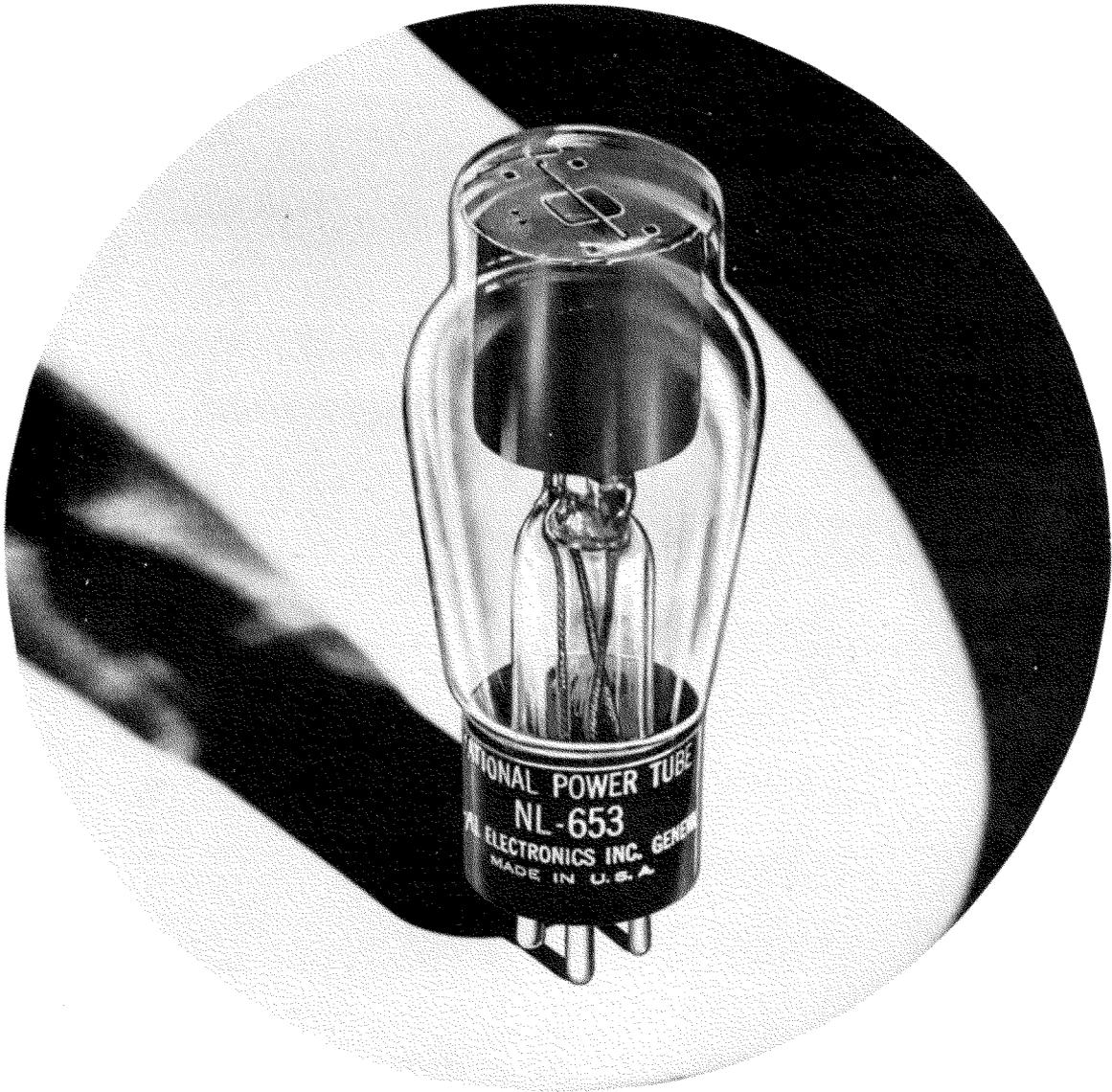
NATIONAL POWER TUBE NL-653 is a sturdy, single-ended, rectifier tube designed especially for industrial power rectifier applications and for "back-rectifier" applications in conjunction with a thyatron tube. It is mercury filled for efficiency, long life, and the ability to stand high inverse voltage.
