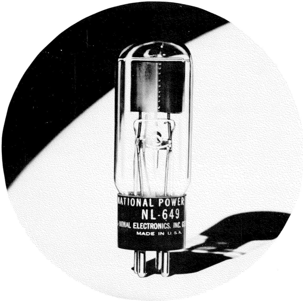
NATIONAL POWER TUBE NL-649 is a sturdy, single-ended, rectifier tube designed especially for industrial power rectifier applications and for "back-rectifier" applications in conjunction with a thyatron tube. It is mercury filled for efficiency, long life, and the ability to stand high inverse voltage.
