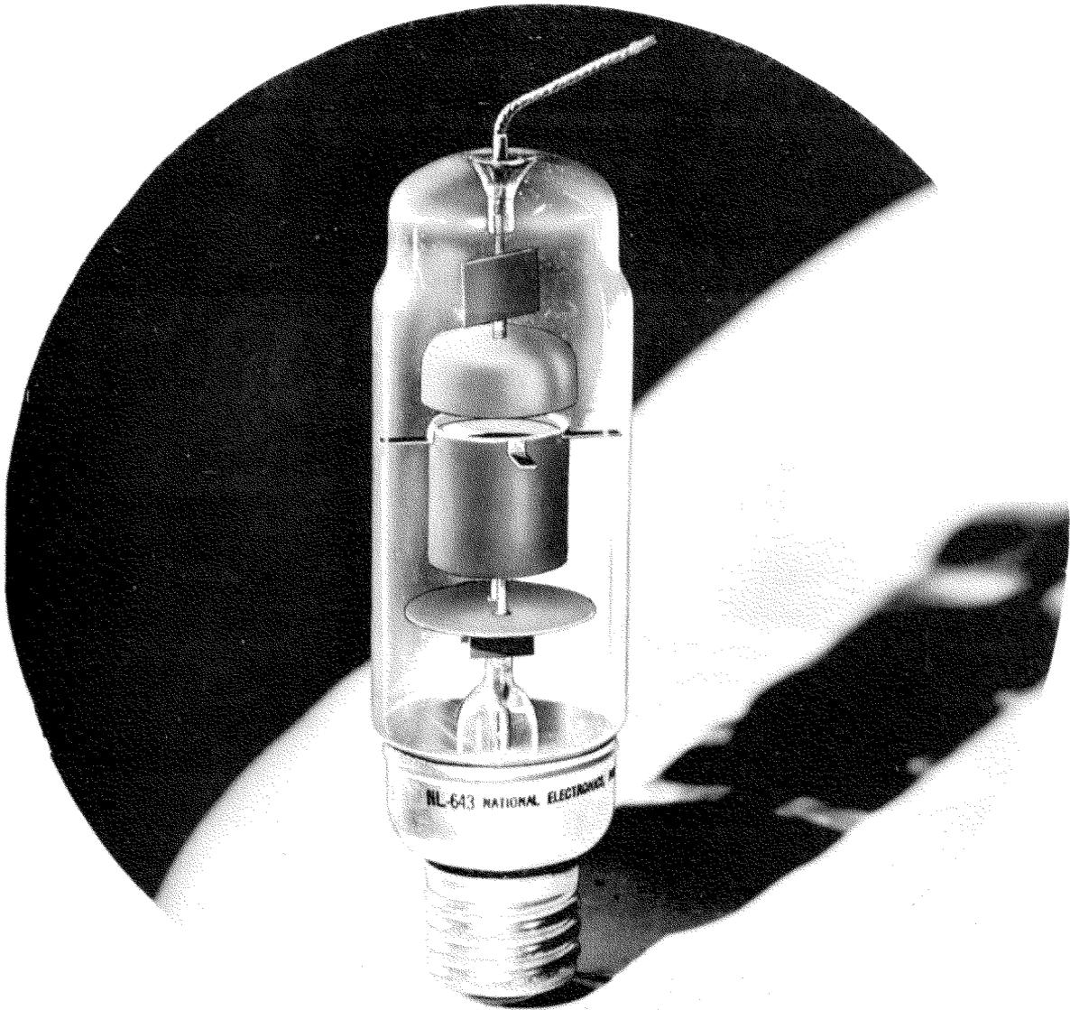
NATIONAL POWER TUBE NL-643 is a sturdy rectifier tube designed especially for industrial power rectifier applications up to 200 volts dc. It is mercury filled for efficiency and the ability to withstand high inverse voltage. NL-643 is designed to give exceptionally long life when used within its ratings.
