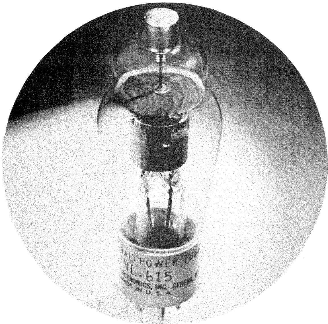
NATIONAL POWER TUBE NL-615 is a sturdy rectifier tube designed especially for industrial power rectifier applications up to 600 volts dc. It is mercury filled for efficiency, long life, and the ability to stand high inverse voltage.
