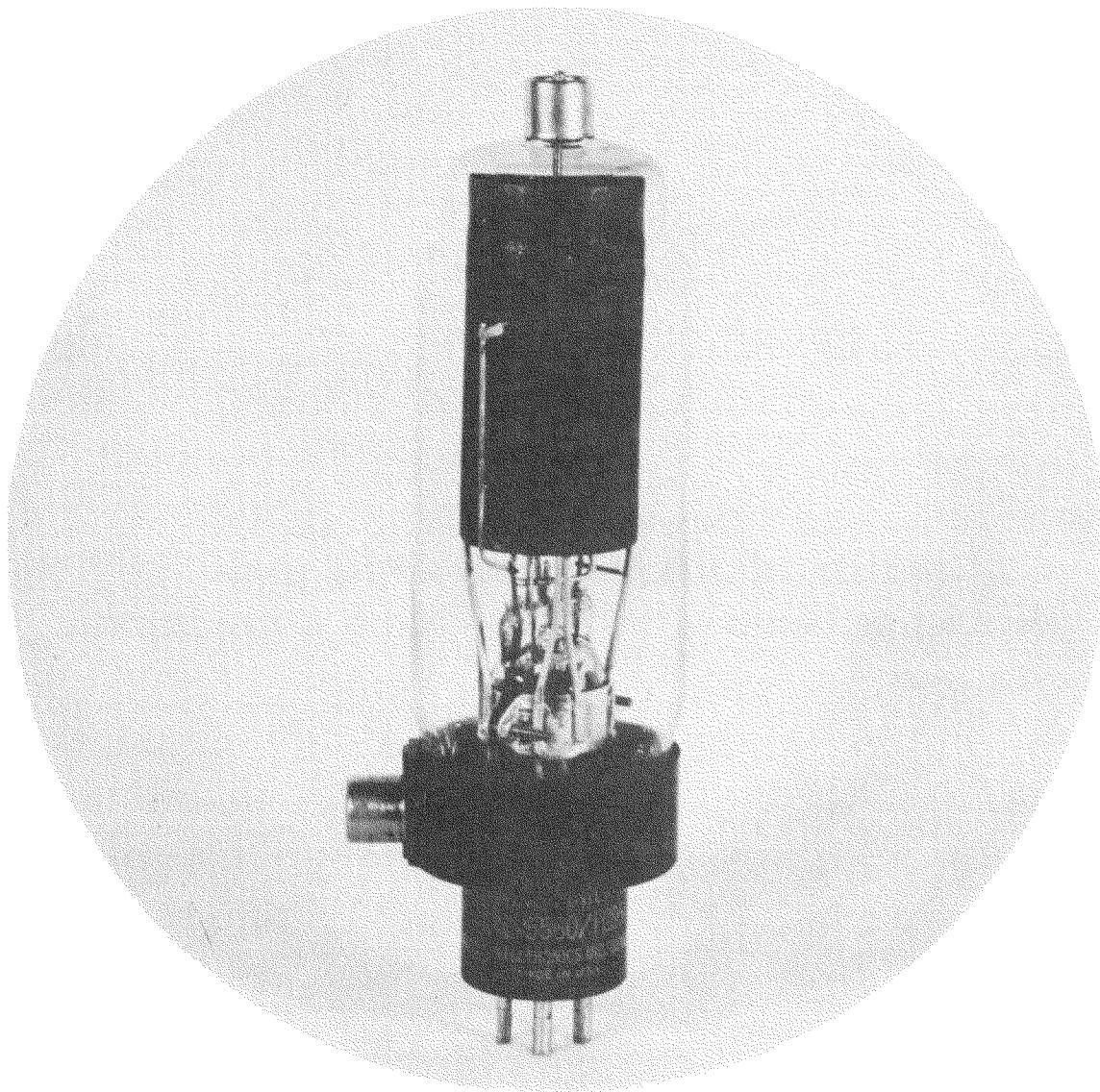
NATIONAL POWER TUBE NL-5560/FG95 is an indirectly heated cathode thyatron designed especially for control, timing, and ignitor firing applications. The shield grid construction and mercury vapor filling give stable operation even with high impedance grid supplies.
