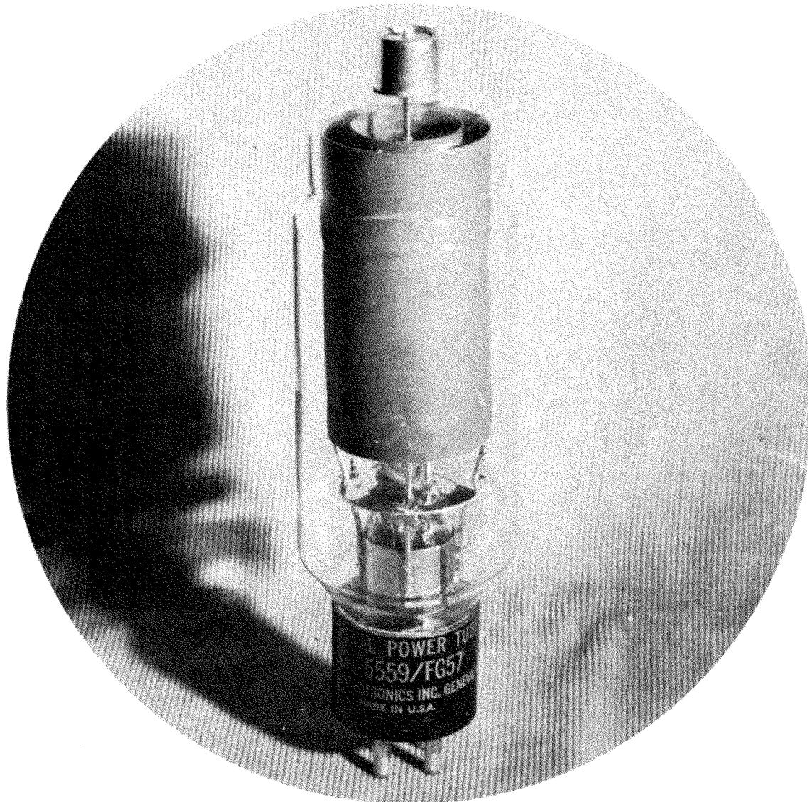
NATIONAL POWER TUBE NL-5559/FG57 is an indirectly heated cathode thyratron designed especially for those applications where little grid power is available. The mercury filling and efficient cathode give long and dependable life.
