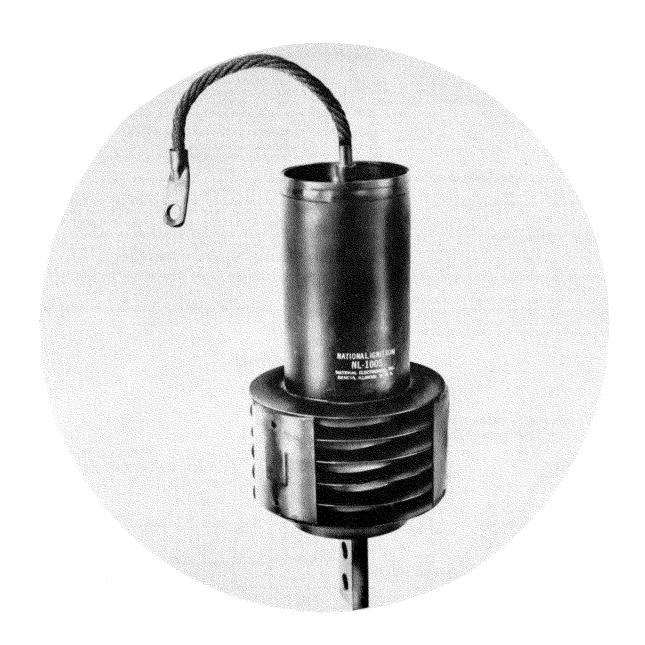
NATIONAL IGNITRON NL-1005 is a sturdy, metal, air-cooled mercury pool tube designed especially for welder control and similar AC control applications. It is also useful in some rectifier applications. NL-1005 is designed for forced air cooling but may be used with free air cooling at reduced ratings.
