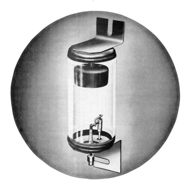
NATIONAL IGNITRON NL-1001 is a sturdy, glass, air-cooled mercury pool tube designed especially for welder control and similar AC control applications. It is also useful for demonstrating the operating principles of ignitors and ignitrons. NL-1001 is designed for forced air cooling but may be used with free air cooling at reduced ratings.
