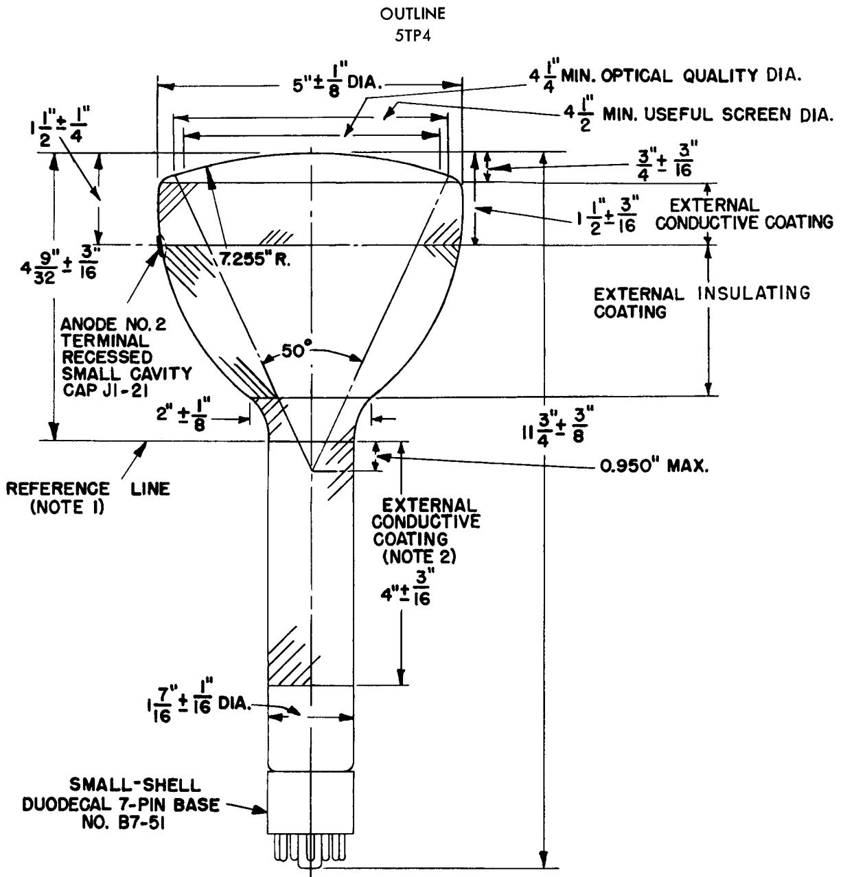
ANODE-NO.2 TERMINAL ALIGNS WITH VACANT PIN-
