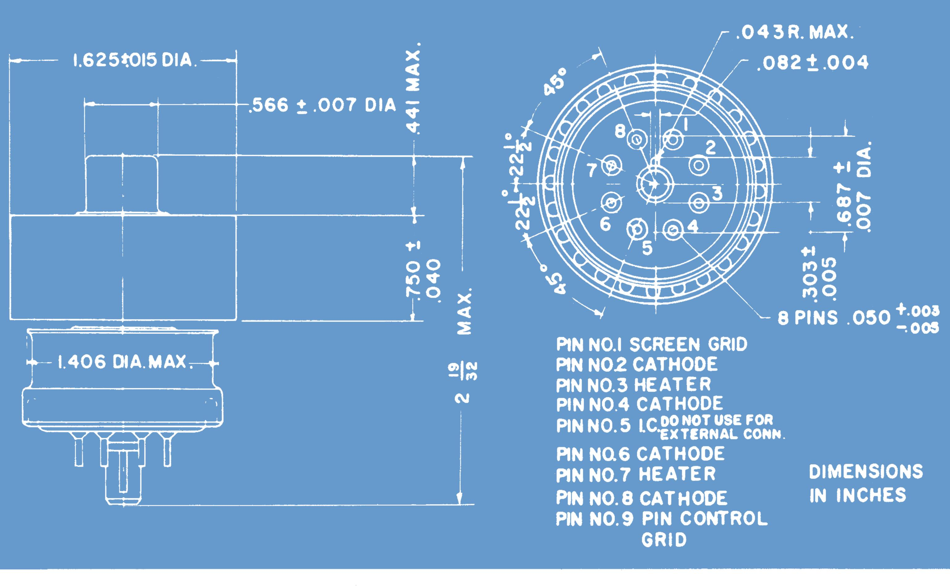
The Eimac 4X250B is a compact, oxide-cathode, external-anode power tetrode, unilaterally interchangeable with the 4X150A in nearly all cases, and is intended for use as an amplifier, oscillator or frequency multiplier over a wide range of frequencies extending into the UHF region. It is cooled by convection and forced air.
