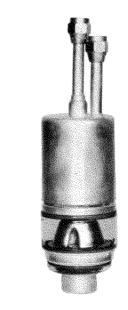
The water-cooled anode requires one gallon of cooling water per minute for the rated plate dissipation of 5 kilowatts. The outlet water temperature must not exceed a maximum of 70°C. under any conditions. The inlet water pressure must not exceed a maximum of 60 pounds per square inch. The pressure drop across the anode is negligible compared to the drop in the associated piping.
