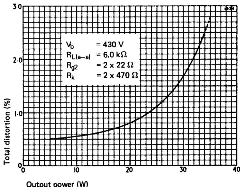
**Triode connection. Push-pull. Class AB1. Cathode bias.**
