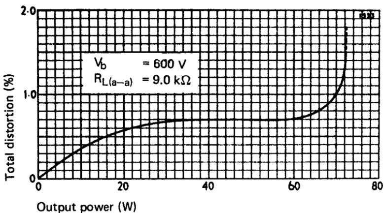
**Ultra-linear connection. 43% taps. Push-pull. Class AB1. Cathode bias.**
