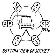
The RK-49 is a heater type aligned grid beam power amplifier tube having an isolantite base. The use of aligned grids reduces the ratio of screen current to plate current and allows more efficient utilization of the total space current. The electrical characteristics are similar to those of the type 6L6G.
