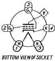
The RK-39 and RK-41 are heater type aligned grid beam power amplifier tubes having isolantite bases. The use of aligned grids reduces the ratio of screen current to plate current and allows more efficient utilization of the total space current. The deflector plates in the RK-39 and RK-41 are connected internally to the cathode.
