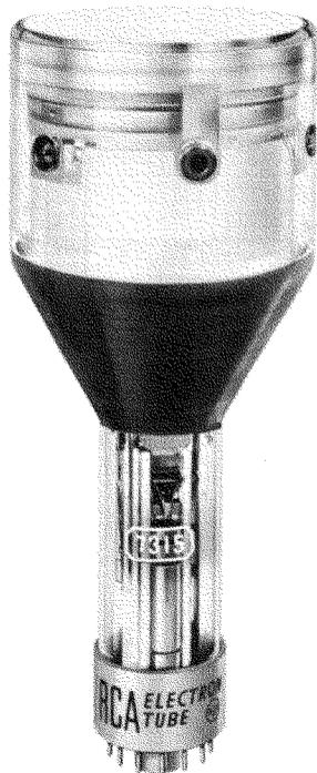
Performance of the 7315 when operated with 10,000 volts on the screen is characterized by a 3.8-inch-diameter display having brightness of about 2750 foot-lamberts; good resolution capability in half-tone displays; and
