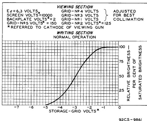
Fig.4 - Typical Storage-Grid Characteristic of Type 7315.
