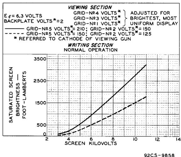
Fig.3 - Typical Characteristics of Type 7315.
