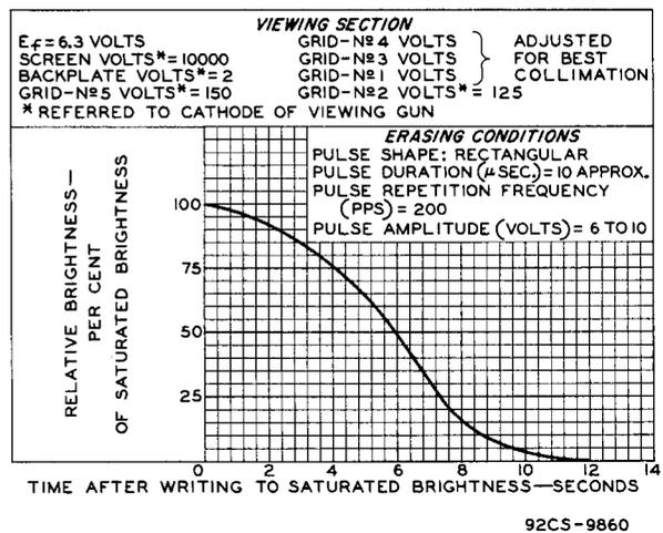
Fig.5 - Typical Erasure Characteristic of Type 7315.
