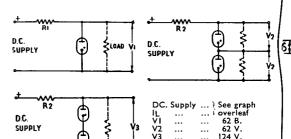
Because of the constancy of ignition voltage this valve can readily be employed in voltage overload protection devices for instruments, etc.
