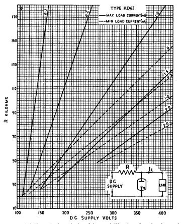
This graph facilitates the determination of the permissible values of supply voltage and series resistance for operation with various loads permanently connected in parallel with the KD63.
