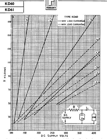
This graph facilitates the determination of the permissible values of supply voltage and series resistance for operation with various loads permanently connected in parallel with the Stabiliser Valve.
