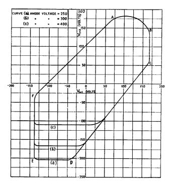
It should be noted that the above quadrant diagram is for an average EN30 and due allowance should be made for trigger voltage tolerance (see pagel).
