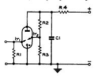
The recommended method of triggering is to apply a positive voltage to trigger electrode No. 2 ( $tr_2$ ) and a negative pulse to trigger electrode No. 1 ( $tr_1$ ).
