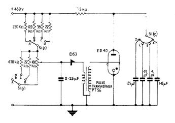
The  $7\cdot 5~k\Omega$  charging resistor should be preferably of the vitreous type with a dissipation rating of 14 watts.
