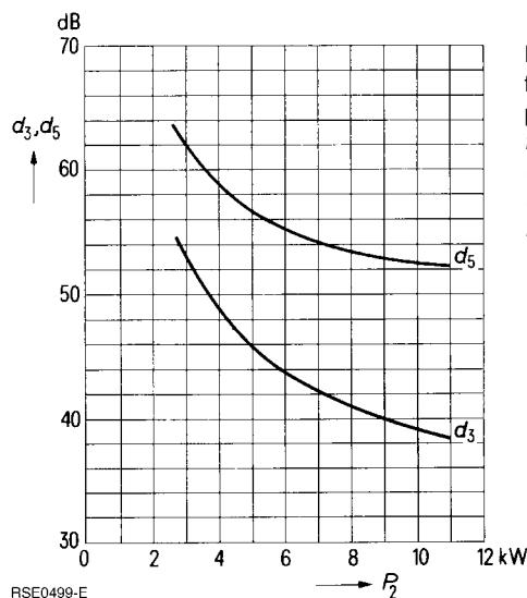
Level of non-linear cross talk resulting from third and fifth order intermodulation products as measured by the 2-tone method at  $f = 30$  MHz,
