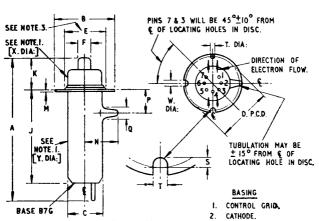
NOTE, I, THIS PORTION OF BULB WILL NOT FOUL A CYLINDER OF INT: DIA: SPECIFIED WHICH IS CONCENTRIC WITH THE PITCH CIRCLE OF THE LOCATING HOLES IN DISC.
