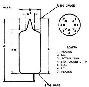
DENOTES:- MEASURED FROM BASE SEAT TO BULB TOP LINE, AS DETERMINED BY RING GAUGE OF E' INT: DIA.
