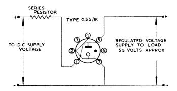
TYPICAL CIRCUIT TO PROVIDE A REGULATED SUPPLY VOLTAGE REMOVAL OF THE VALVE FROM THE SOCKET DISCONNECTS THE VOLTAGE FROM THE LOAD
