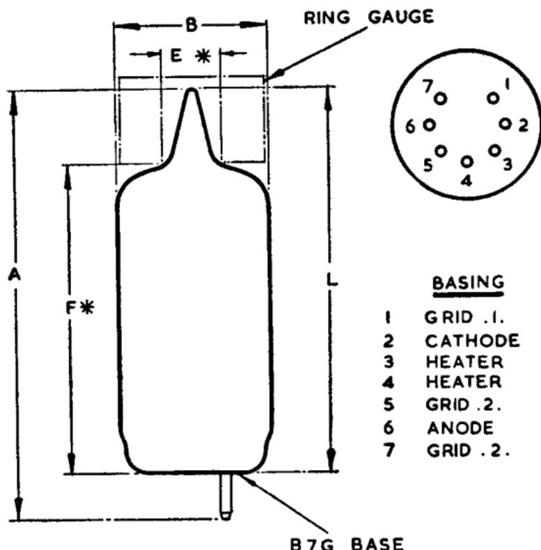
\* DENOTES:- MEASURED FROM BASE SEAT TO BULB TOP LINE, AS DETERMINED BY RING GAUGE OF 'E' INT. DIA.
