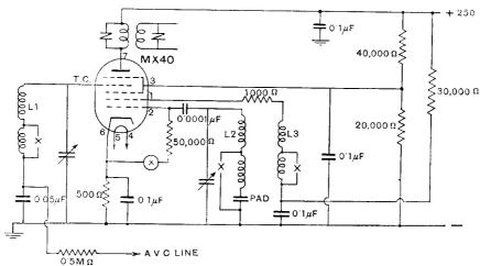
THE COUPLING BETWEEN L2 & L3 SHOULD BE ADJUSTED UNTIL A MILLIAMMETER INSERTED AT THE POINT (X) IN SERIES WITH THE GRID LEAK CIVES A READING OF 0'2 MILLIAMPERES
