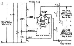
$c_1=$  FILTER CONDENSER  $c_2$  ,  $c_3$  ,  $c_4=$  SEE NOTE 3  $R_1+R_2+R_3+R_4=$  BLEEDER POTENTIOMETER  $R_1=0.200$  MEGOHM  $R_2=0.200$  MEGOHM  $V=V_0$  V = VOLTMETER  $V=V_0$
