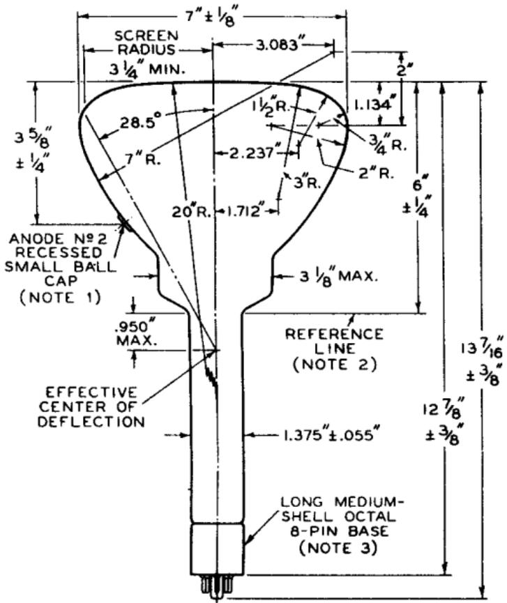
**NOTE 1:** THE PLANE THROUGH THE TUBE AXIS AND PIN No. 2 MAY VARY FROM THE PLANE THROUGH THE TUBE AXIS AND ANODE No. 2 TERMINAL BY AN ANGULAR TOLERANCE (MEASURED ABOUT THE TUBE AXIS) OF  $10^\circ$ . ANODE No. 2 TERMINAL IS ON SAME SIDE OF TUBE AS PIN No. 2.
