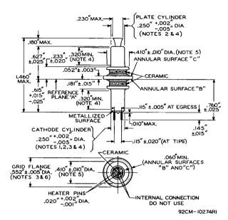
REFERENCE PLANE "A" IS DEFINED AS THAT PLANE AGAINST WHICH ANNULAR SURFACE "B" OF THE GRID FLANGE ABUTS.
