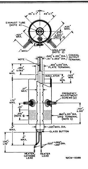
NOTE 1: THE AXES OF THE INNER AND OUTER CONDUCTORS OF THE COAXIAL OUTPUT TERMINAL COINCIDE WITHIN 0.010".
