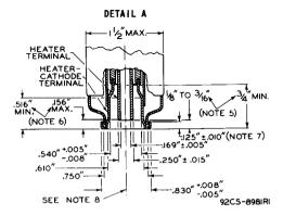
REFERENCE PLANE A IS DEFINED AS THE PLANE THROUGH THAT PORTION OF THE MOUNTING FLANGE DESIGNATED AS ANNULAR SURFACE D.
