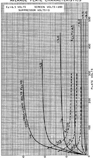
PLATE (Ib) OR SCREEN (IC2) MILLIAMPERES
