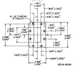
Reference plane I is defined as that plane against which the waveguide output flange abuts.
