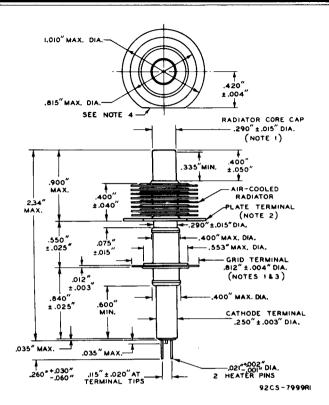
NOTE 1: ECCENTRICITY OF RADIATOR-CORE CAP WITH RESPECT TO THE CATHODE TERMINAL IS ONE-HALF THE TOTAL RUN-OUT DETERMINED BY CHUCKING THE CATHODE TERMINAL 0.050" TO 0.100" FROM CATHODE FLANGE, ROTATING THE TUBE, AND GAUGING THE TOTAL RUN-OUT AT A POINT 0.125" FROM THE END OF THE RADIATOR-CORE CAP. THE ECCENTRICITY WILL NOT EXCEED 0.030".
