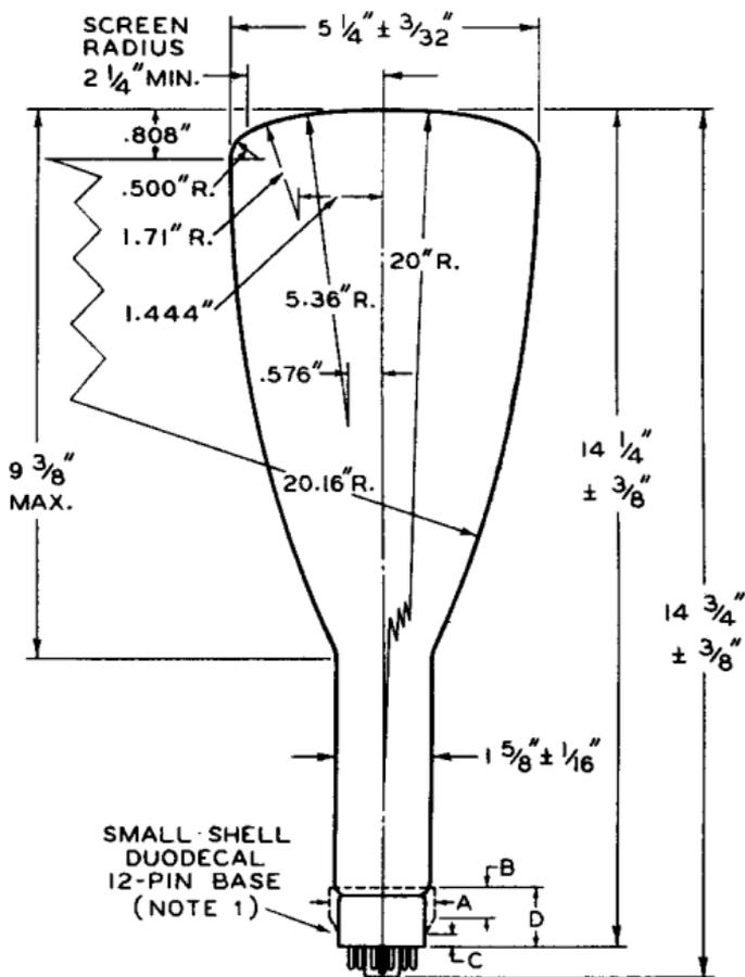
∅ OF BULB WILL NOT DEVIATE MORE THAN 2° IN ANY DIRECTION FROM THE PERPENDICULAR ERECTED AT THE CENTER OF BOTTOM OF THE BASE.
