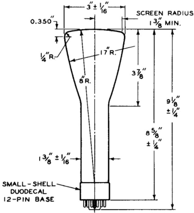
AXIS OF BULB WILL NOT DEVIATE MORE THAN  $2^{\circ}$  IN ANY DIRECTION FROM PERPENDICULAR ERECTED AT CENTER OF BOTTOM OF BASE.
