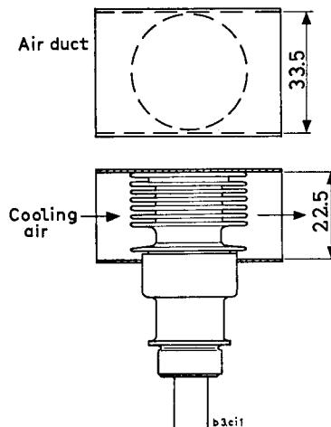
The eccentricity of the contact surfaces is max. 0.5 mm
