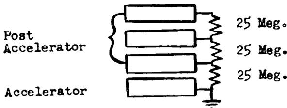
The two accelerator terminals must be connected together.
