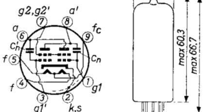
Low loss socket without collar is recommended. At high frequencies use of a metal retaining device is not recommended due to loss of output power
