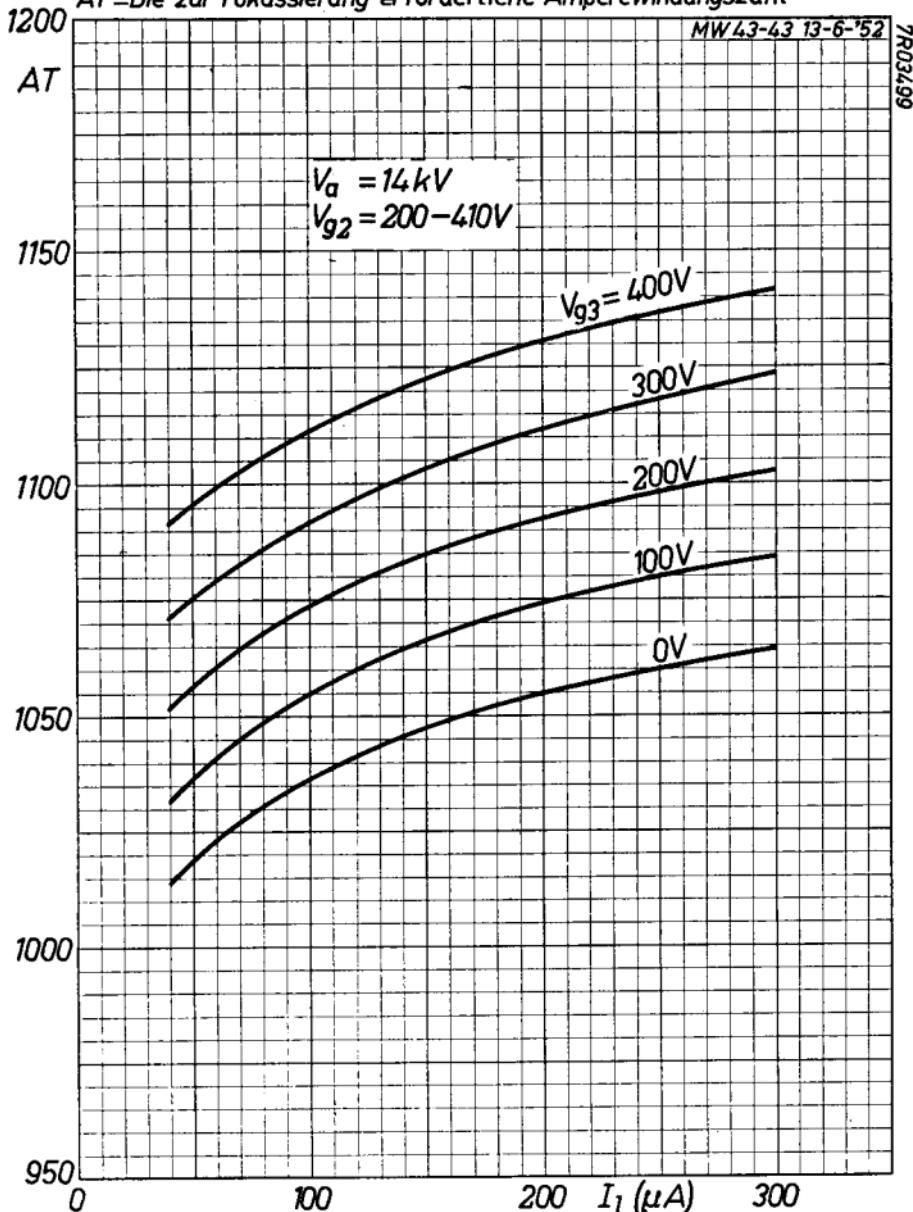
AT=Number of ampere turns necessary for focusing
