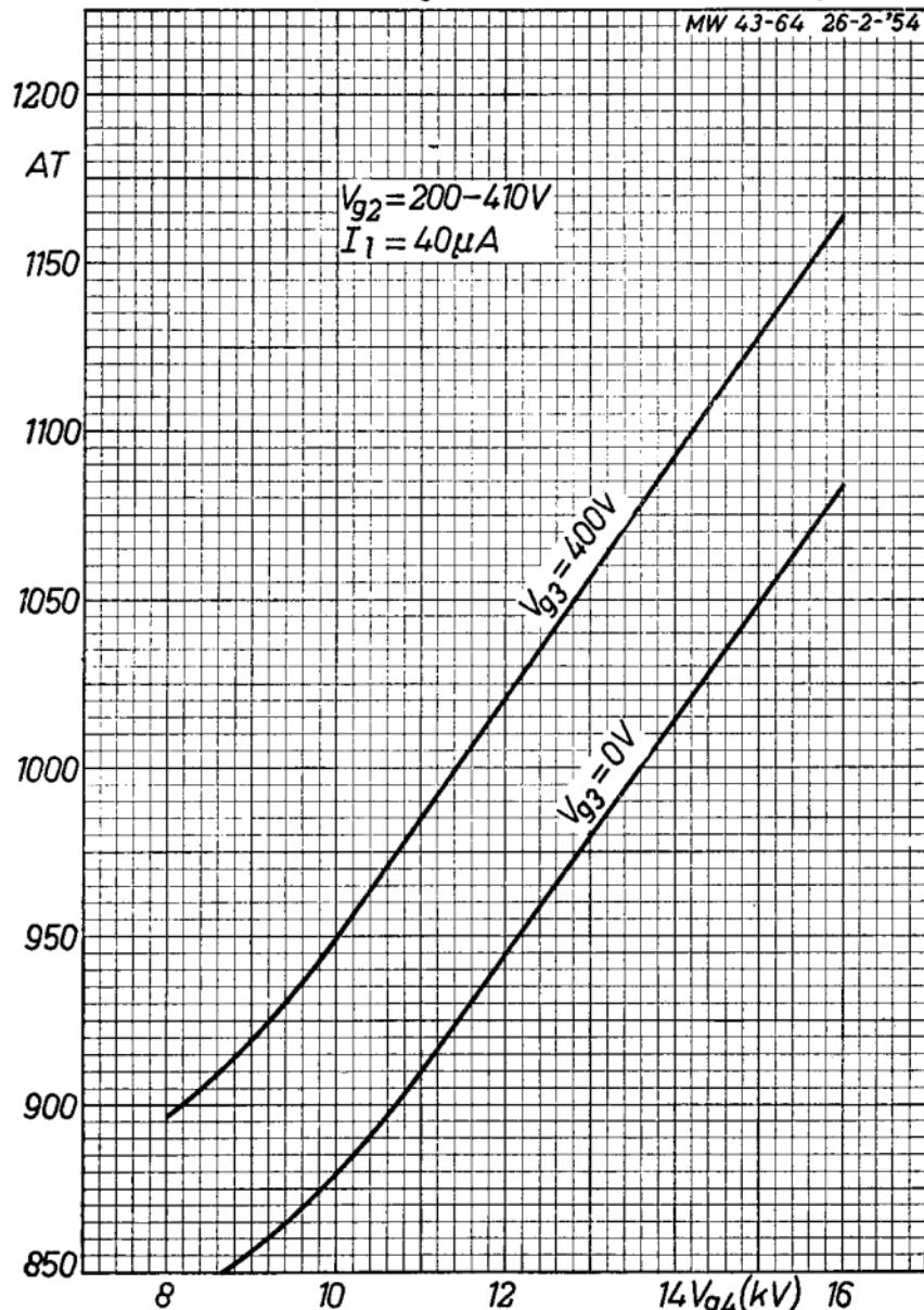
AT=Number of ampere turns necessary for focusing
