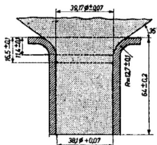
Remark: Any material in contact with the cone or the face must have insulating properties adequate for 16 kV
