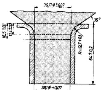
Reference line gauge. The inner surface of the coils must not extend into the shaded region.
