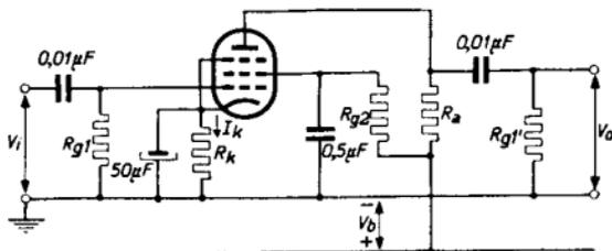
This tube can be used without special precautions against microphonic effect in amplifiers in which the input voltage  $V_i \geq 5$  mV for maximum output of the output tube and in receivers in which  $V_i \geq 0,5$  mV for an output of 50 mW
